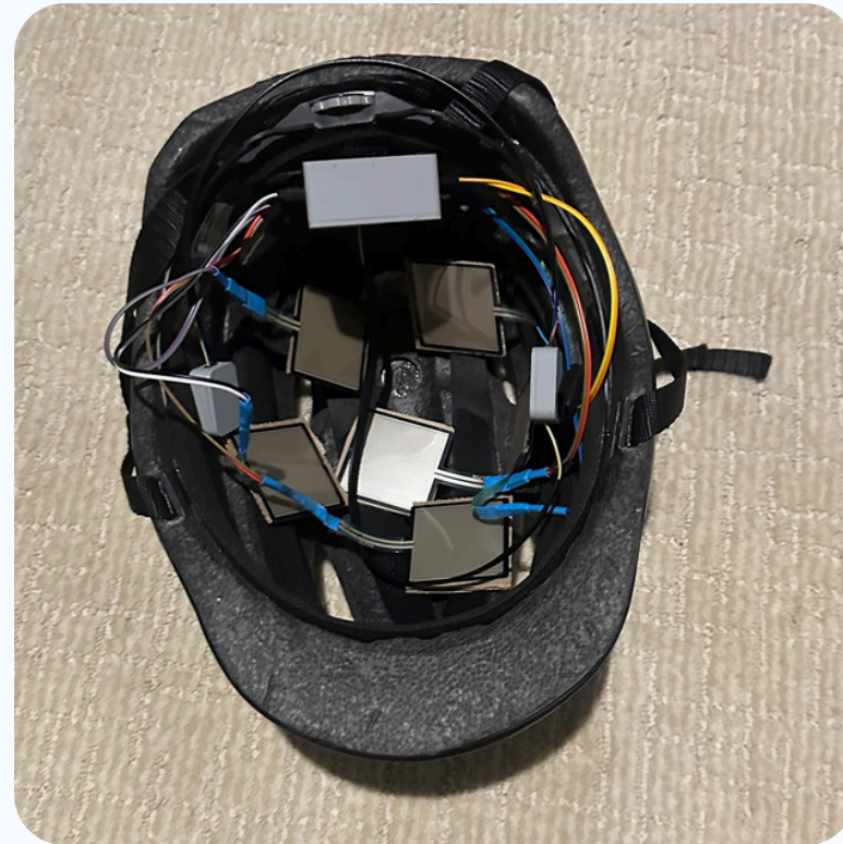
Feasibility prototype that includes accelerometers & FSRs
